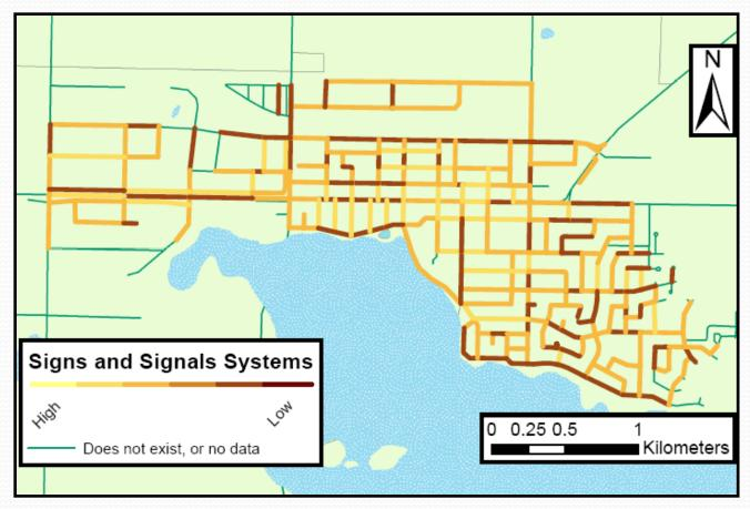
Presence of traffic signs and signals indicates a higher level of traffic safety.
